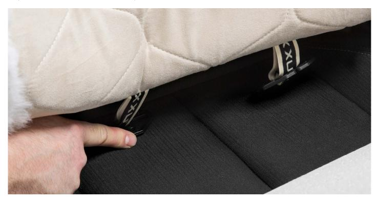
⑥ Secure the hooks at the bottom of the seat cover to the underside of the seat. Be sure NOT to connect the hooks to any wiring, electrical components or mechanisms used to move the seat forward, backward, up or down.
