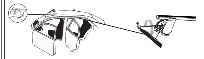
Insert the two lugs on the side of the front cover into the leg, using the key provided turn the lock barrel to the open position (O), engage the locking tab into the leg and turn to lock. Refer instruction 14 below for lock positions.
