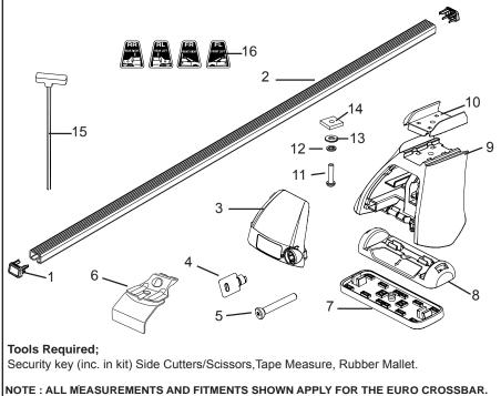
NOTE: Refer to the DK Specification sheet for correct placement (Front or Rear, Left or Right) of the FOOT PLATE, RUBBER PAD and METAL STRAP. Also refer for sizes to cut the BAR MEASUREMENT STRIP.
