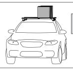
70kg load rating (Urban road) = 35 kg load rating (Off road - 70kg / 2)
