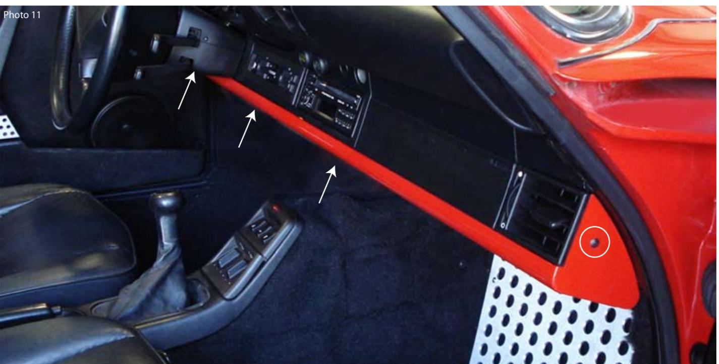
Step 12: Using the (2) supplied .5" button head screws, nuts and washers attach the bottom of the dash panel into the factory holes on the drivers side and center of the dash.
