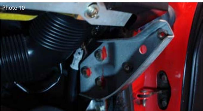
Installing the Rennline lower dash delete panel.
