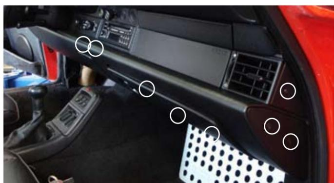
Step 3: Remove trim piece around radio by simply prying it off. Lift retaining bar on both sides of the radio as shown in photo 3 and pull radio out.
