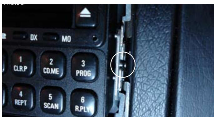
Step 5: Remove the end bolts (both sides) as shown in photo 5. Also, remove the 2 bolts in the center located in the ashtray area.
