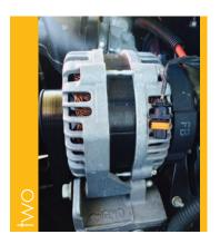
2. To test the F terminal (with the ignition off) unplug the voltage regulator connector.
