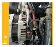
4. Connect a test lamp to B+ and probe the voltage regulator harness at the F terminal.
