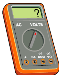
Usage of a voltmeter is not an accurate test, due to the slow refresh rate.
