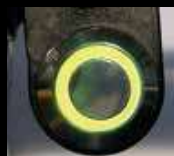
LED loop YELLOW valve 40% open
