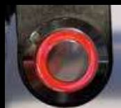
LED loop RED valve 100% open
