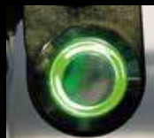
LED loop GREEN valve 10% open
