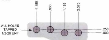
USE OF HIGH STEER IS OPTIONAL AND REQUIRES CUSTOM STEERING LINKAGE AND TRACK BAR RE-LOCATION. If not using high-steer arms, you may wish to plug the high steer threaded holes with short 1/2" x 20 bolts to preserve the threads for future use. Reid Racing knuckles have been machined and drilled for use with high steer arms, all angle correction has been machined directly into the knuckle so simple flat arms can be manu-factured.
