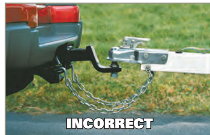
Trailer not level
