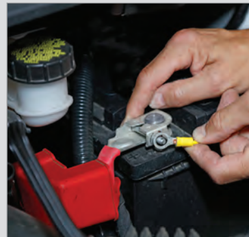
NOTE: Some vehicles may require grounding and/or direct connection to the battery.
