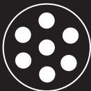
7-Pin Round Turn, Stop, Tail, Electric Brakes, Auxiliary, Ground
