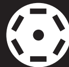
7-Way Blade Turn, Stop, Tail, Electric Brakes, Auxiliary, 12V, Ground
