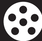
6-Pin Round Turn, Stop, Tail, Electric Brakes, Auxiliary, Ground
