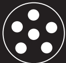
6-Pin Round Turn, Stop, Tail, Electric Brakes, Auxiliary, Ground
