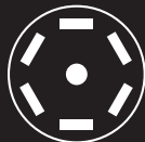
7-Way Blade Turn, Stop, Tail, Electric Brakes, Auxiliary, 12V, Ground
