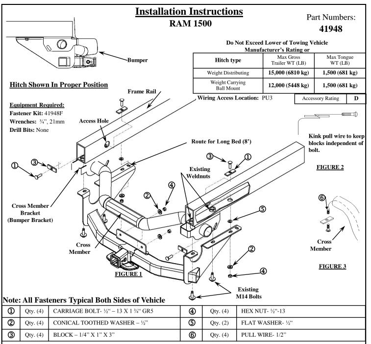
Removal of the spare tire will make installation easier.
