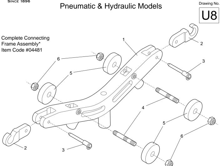
\*Connecting Frame Assembly #04481 does not include part #2 (Chain Hook) & part #3 (Release Pin). These items must be ordered separately. Please refer to chart below.
