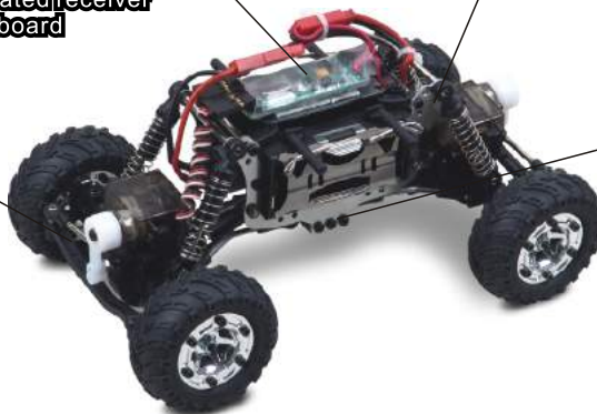
Updated 4-link suspension (bent linkage bar)
