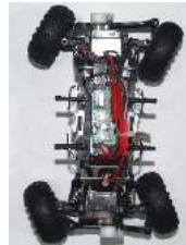
Front/rear wheel steering (In the opposite direction)
