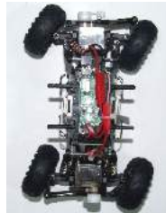
Front/rear wheel steering (In the same direction)
