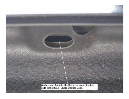
Insert Toggle bolt (with bolt inserted in the reverse direction into wing). This allows one to attach and detach brackets at any time without the bolt head interference. Add a fender washer, homemade aluminum bracket and nut to secure in place.
