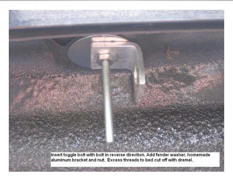
Cut off excess threads. Now you could have inserted the bolt the other way but would have had to use a double nut process to lock the bolt up inside the bedrail. This way allows a secure fit that will never come loose.
