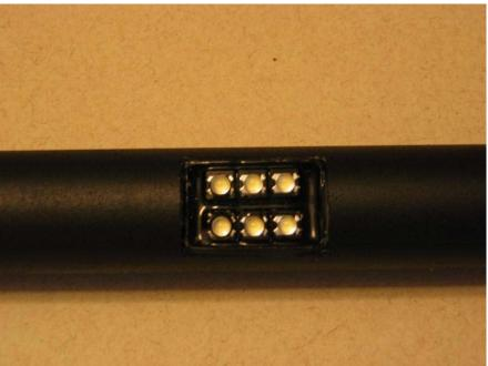
A small hole was drilled in the aft end of the tube to allow the power cord out since the ends will be blocked with the well nuts. Insert the tube into the bracketed well nuts and tighten until tube is snug and does not spin freely. Adjust the angle of the lights so that they point towards the center of the truck bed (best done at night to get optimal lighting situation).
