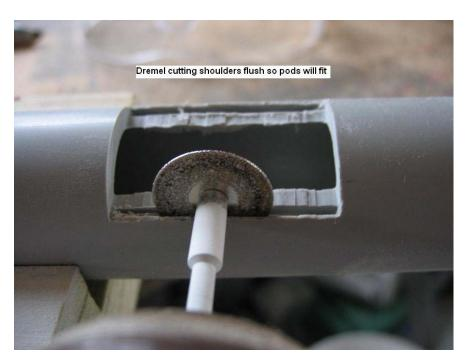
One tube finished with cutting. Make sure you leave room on the ends and don't put the holes too close as you need room for the well nuts to be inserted and expand inside the tube for attachment. You may want to paint the tube at this time. I did it later in the procedure.
