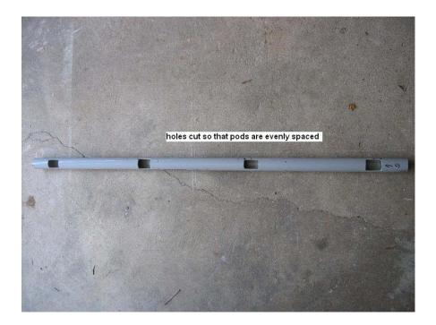
Take one string of Recon bed lights and tape the pods to the holes with lights facing inward. This gives the correct spacing and allows you to fold and zip-tie the excess wiring for a tidy install.
