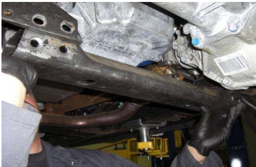
37. Re-install the rear cross member as original.
