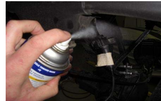
58. Lube the ABS wire and slide the rubber mount to gain more slack.
