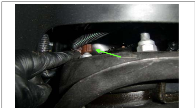
10. Remove the clips from on top of the upper strut mounting nuts.
