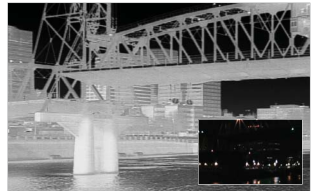
Thermal image of bridge structure at night and what the human sees (inset)
