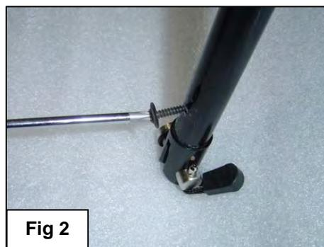
4. Remove clip from pin, then remove pin from Billet Disconnect
