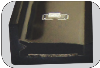
Completely encapsulated circuit board with robotically assembled high intensity LED bulbs
