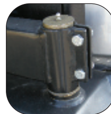
Adjustable, easy swivel hinge with grease fitting.
