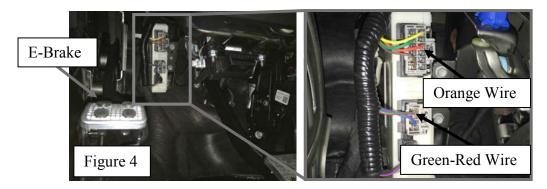
3. Attached 6" wire between Orange wire(Pin 3 on C2498C Connector) and Green-Red wire (Pin 1 on C2498A Connector) using scotchloks. This will activate a continuous +12V to the +12V power pin on the 7pin trailer connector. Refer to **Figure 5**
