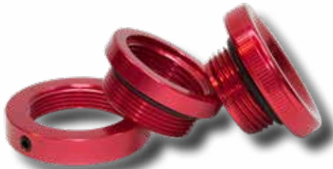
PN 4120452 - MODULAR FILLER CAP, Modular, Billet Aluminum Screw-In Type to Prevent Seepage & Oil Loss, for 1.375" ID Hole, w/ O-Ring Seals, Red Anodized
