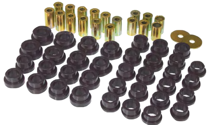
#14-307-BL Nissan 350Z '03-'09 Rear Control Arm, Radius Arm & Lower Link Bushing Set
