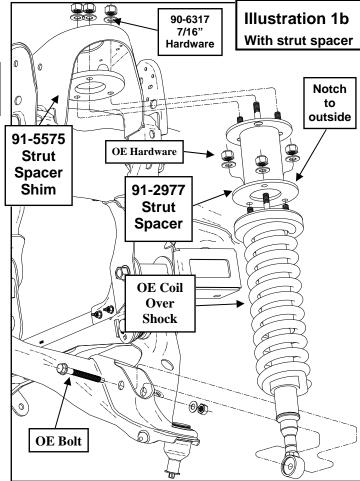
coil-overs have the suspension and headlights re-aligned.
