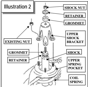
pocket. Remove the coil springs.
