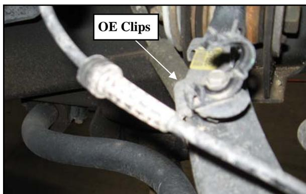
6. Unbolt the brake line bracket from the upper A-arm.
