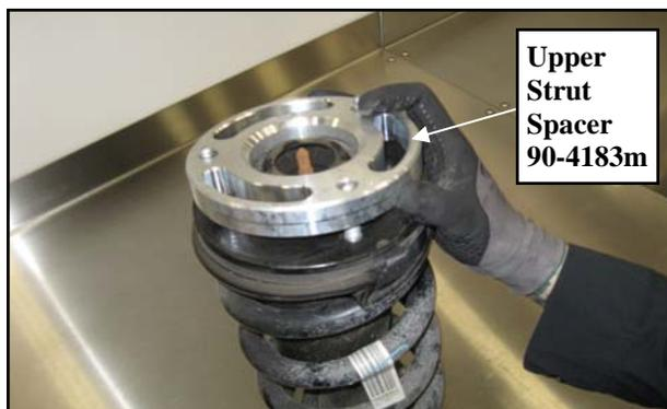
12. Install the strut assembly into the strut tower and secure using the supplied **10mm** flange nuts. Leave the bolts hand tight only at this point.
