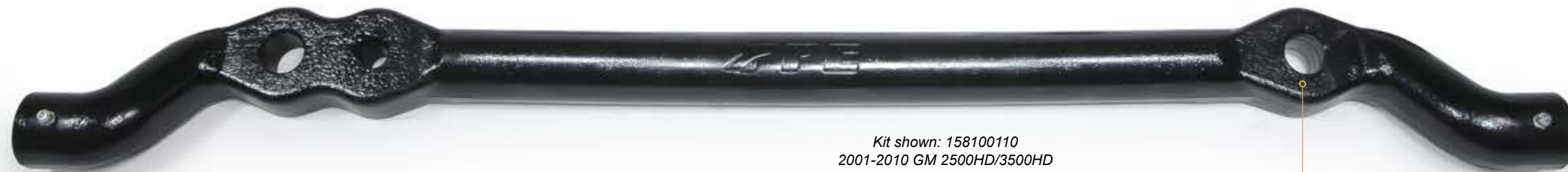
Following the GM design change, PPE incorporated the solid mounting design
