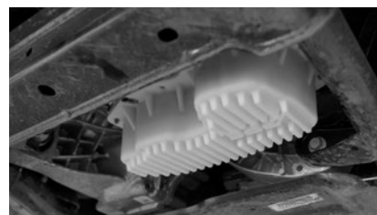
3D printed prototype test fit on vehicle
