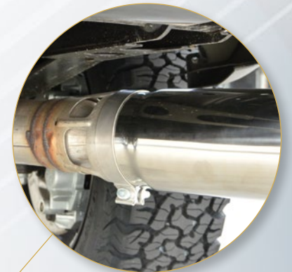
Fits over the stock exhaust tip
