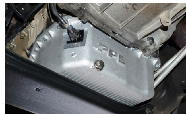
PPE High-Capacity Cast Aluminum Oil Pan Kit comes complete with hardware, pan, NPT plug and billet stainless steel Neodymium drain plug. All you add is RTV sealant and oil.
