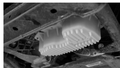
3D printed prototype test fit on vehicle
