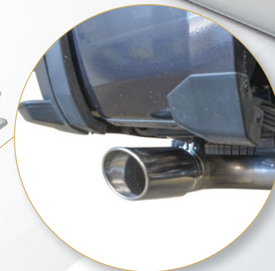
Replaces long, stock, restricted L5P exhaust pipe
