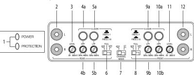
Status LEDs (on top of amplifier): Power and Protection—Power will illuminate to indicate
