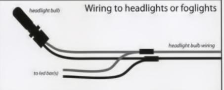
to red wire on led bar to ground wire on battery to constant positive (+)
