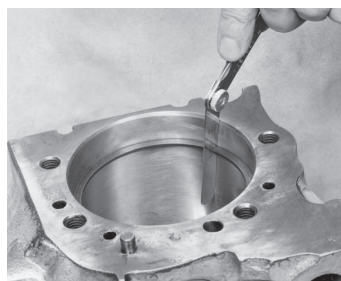
② Measure gap precisely with feeler gauges
