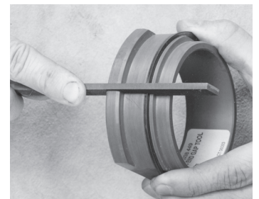
③ Use fixture to hold ring when filing end cap
