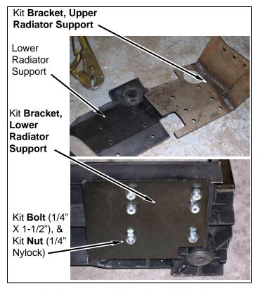
Position and mark holes from kit bracket, upper backing plate on side support as shown. Drill 1/ 4" holes where marked.
