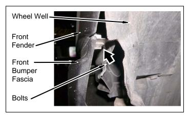
e. Remove six bolts and front bumper fascia from vehicle.
