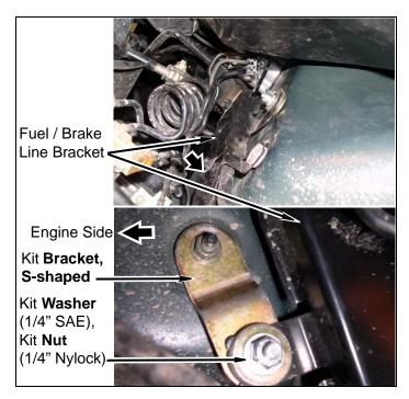
b. Install kit bracket, straight on the wheel well side of the fuel / brake line bracket with a kit washer (1/4" SAE) and kit nut (1/4" nylock) as shown. Install two kit brackets and fuel / brake line bracket on firewall with two nuts.
