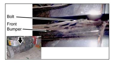
Install front bumper and two kit spacers on front bumper brackets with two kit bolts (M8-1.25 X 40mm). Do not tighten.
