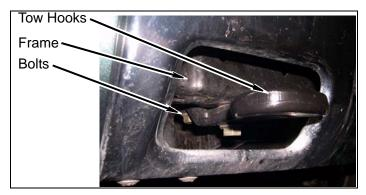
d. Remove four bolts and two side impact braces from frame.
