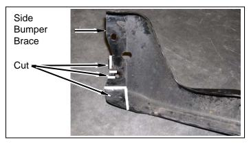
d. Install two side bumper braces onto front bumper with two bolts, two kit **blocks, 2" diameter**, two kit **bolts** (8-1.25 x 90mm), and two kit **washers** (8mm).
