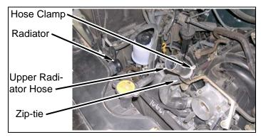
b. Remove three hoses from two fan shroud clips.
