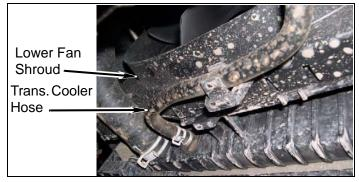
c. Install hose clip, metal transmission cooler hose, and transmission cooler hose on fan shroud and lower fan shroud.
