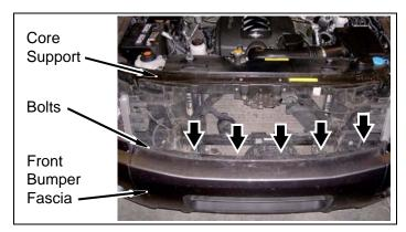
g. Install front bumper fascia onto support with three pop-up clips.
