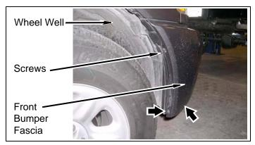
d. Pull driver and passenger wheel well back and remove four bolts from front bumper fascia and front fenders.
