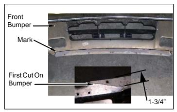
d. Cut front bumper where marked as shown.
