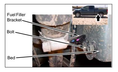
b. Remove fuel cap from fuel filler. Push fuel filler rubber gasket and fuel filler toward inside of bed.
