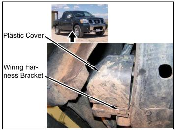
b. Remove bolt and wiring harness bracket from frame.
