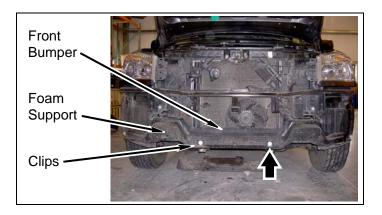
g. Remove six bolts, four nuts, and two side bumper braces from front bumper and side impact braces.
