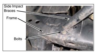
e. Remove four nuts and two side impact braces from front bumper.
