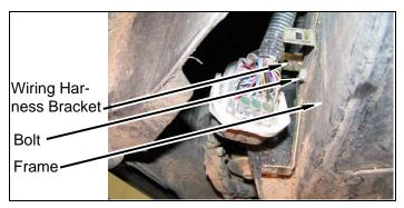
c. Remove two wiring harness push clips and wiring harness from frame / body mount perch.
