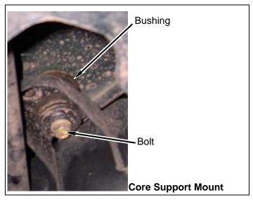
b. Remove three bolts from cab bushings on passenger side.
