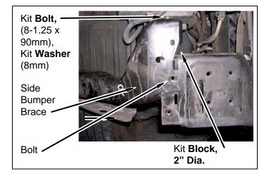
e. Install two side impact braces onto two side bumper braces with four nuts.
