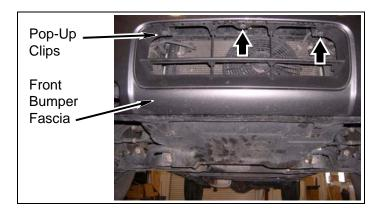
h. Install front bumper fascia onto front fenders with four bolts.
