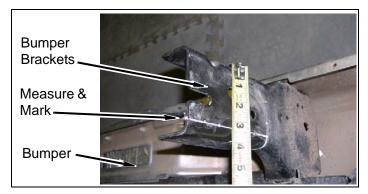
b. Measure and mark a line 6" back from the front of the bumper brackets as shown.
