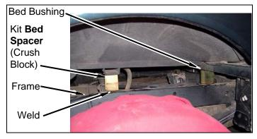
Tack-weld four kit **bed spacers** (crush blocks) to frame.
