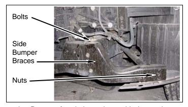
h. Remove four bolts and two side impact braces from frame.
