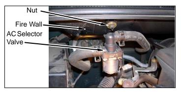
b. Remove nut and AC line bracket from fire wall.
