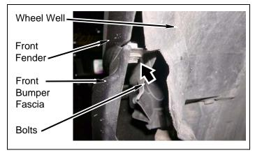
i. Install front bumper fascia onto driver and passenger wheel wells with six screws.
