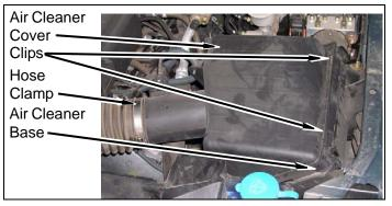
d. Install push clip and wire harness on air cleaner cover.
