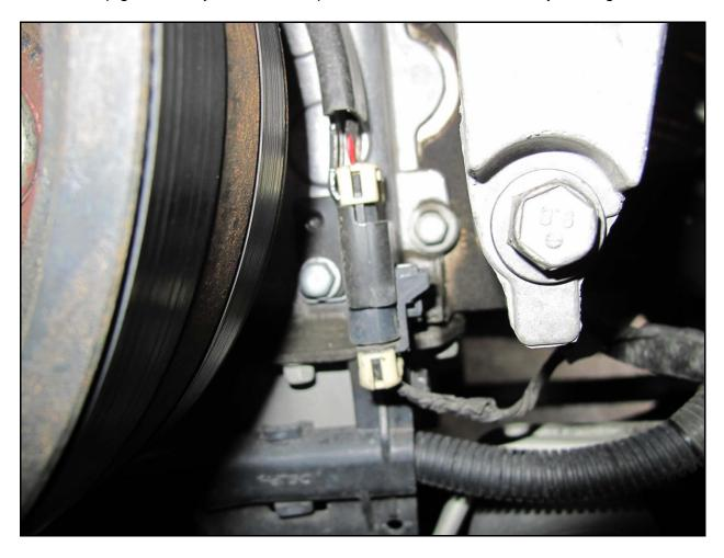
On the driver side of the engine block you will find a black, two pin knock sensor. From the main break out of the Painless harness located at the center-back of intake manifold find the two wire mating connector for this knock sensor. It is labeled DRVR KNOCK and has a grey and blue wire in it. Plug this connector into the driver side knock sensor. Make sure to route the wires so when you install the exhaust headers or manifolds it does not come in contact with them.
