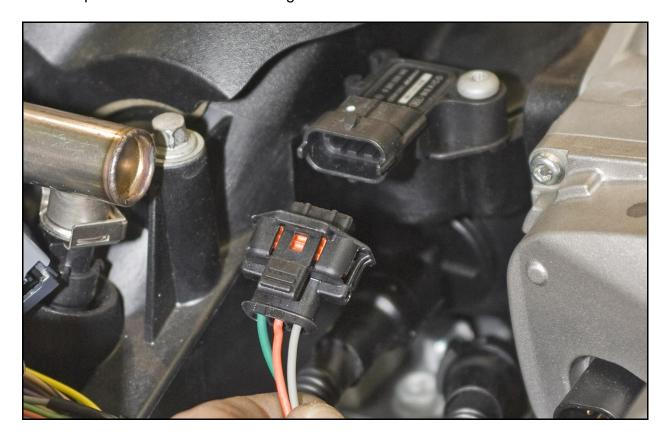
If you have the factory installed fresh air intake from the donor vehicle you should have then also gotten the mass air flow sensor. It should look something like what is shown below. Route the m.a.f. connector over to the m.a.f. sensor and plug it in.
