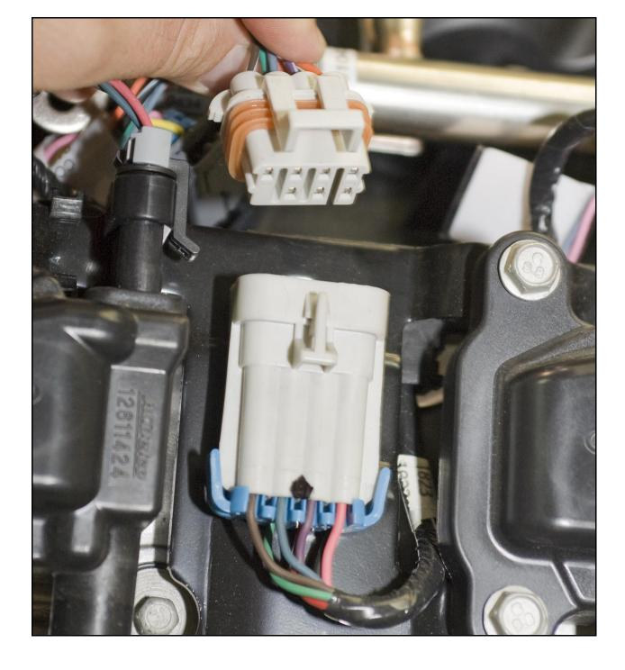
Route the throttle body connector over to the throttle body. Plug it in as shown below.
