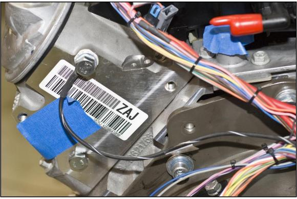
Now work your way down the drive side fuel rail and connect the fuel injector connectors to their corresponding fuel injector. From the front of the engine the injectors are numbered as 1, 3, 5, and 7. Then plug in the driver side coil connector into the coil near plug sub-harness.
