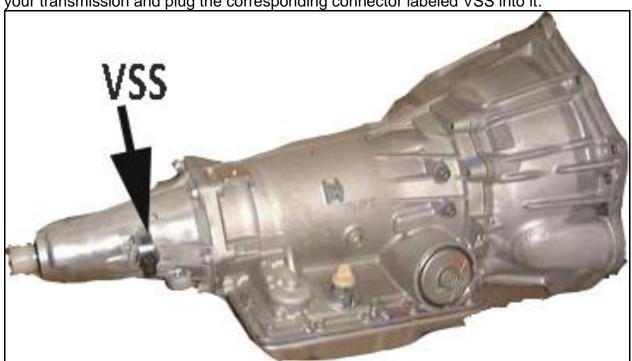
4L80E and 4L85E transmissions have a vehicle speed sensor and also an input speed sensor located on the driver side of the transmission. Below is a picture of a 4L80E transmission for reference. This harness does not support the use of the 4L80E transmission. And we do not have the programming for the use of this transmission at this time.
