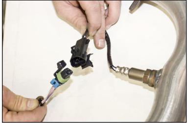
Always install oxygen sensors as close to the engine as possible. Most aftermarket headers come with oxygen sensor bungs already welded into the header collectors.
