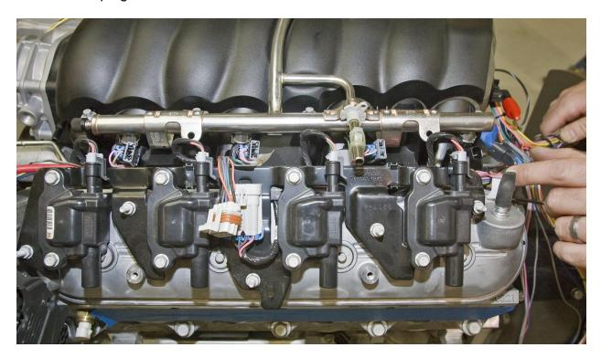
Route the coolant temperature sensor connector to the sensor located right in front of #1 cylinder exhaust port. Plug it in to the sensor.
