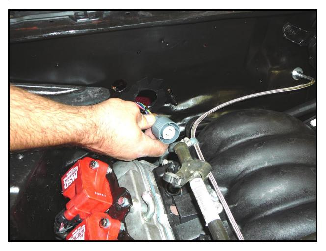
If you chose to mount the ECM, TCM and fuse block in the engine compartment then just route the engine and transmission sections of the harness over towards the centerback of the intake manifold.
