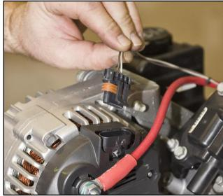
Route the cam position sensor connector down the front of the engine and over to the cam position sensor. You will find this connector has three pins. The Painless harness has an adapter pigtail plugged into it that adapts the harness to match up to the three pin cam position sensor connector on your engine. Plug the three pin connector on the end of this pigtail directly into the cam position sensor connector on your engine.
