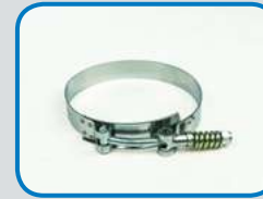
C3875 SPRING LOADED Min: 3.75" [95.3 mm] Max: 4.063" [103.2 mm] Band width: 0.75" [19.1 mm] SAE: 92
