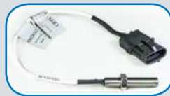
C50032 MAG PICK UP HALL EFFECT SENSOR LENGTH: 2" [50.8mm] THREAD: 3/8 - 24 UNF
