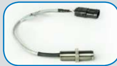
C50279 MAG PICK UP HALL EFFECT SENSOR LENGTH: 2.5" [63.5mm] THREAD: 5/8 - 18 UNF
