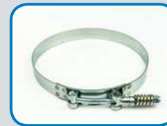
C3883 SPRING LOADED Min: 5.688" [144.5 mm] Max: 6.0" [152.4 mm] Band width: 0.75" [19.1 mm] SAE: 154
