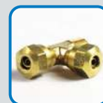
C11795 MALE PIPE RUN TEE Material: Brass Fitting End A: ¼" OD Tube Nylon Fitting End B: ¼" OD Tube Nylon Fitting End C: ⅜" (-2) NPT Male DOT
