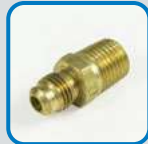
C10770 MALE PIPE CONNECTOR Material: Brass Fitting End A: 1/4" (-4) SAE 45° Male Fitting End B: 1/4" (-4) NPT Male
