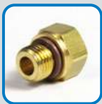
P55116 FEMALE PIPE CONNECTOR Material: Brass Body, FKM Seal Fitting End A: M14 X 1.5 ISO 6149-3 Male Fitting End B: ⅜" (-2) NPTF Female
