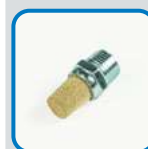
C10774 POROUS BRONZE AIR SILENCER Material: Bronze/Steel Fitting End A: ⅜" (-2) NPTF Male Max Rated: 5 SCFM @ 90 psi
