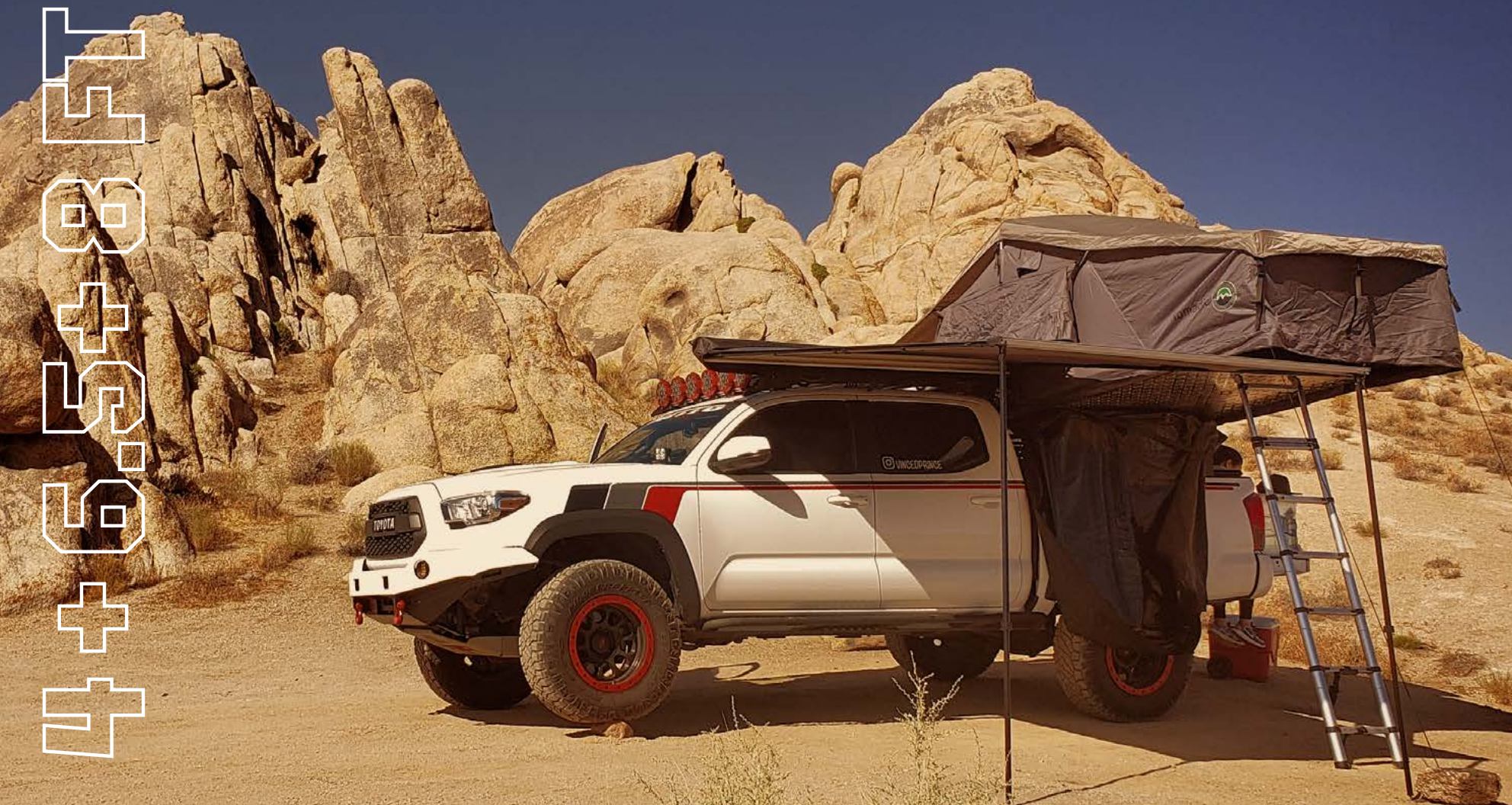
Pivoting aluminum support poles feature twist and lock technology adjustable up to 8.5 feet
