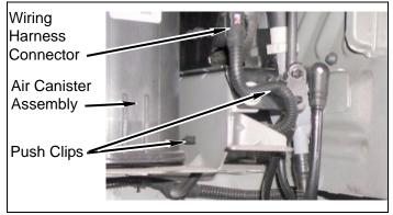
e. Install cover plate on body and air canister assembly with four bolts and one nut.
