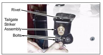
b. **YJ Only:** Remove five bolts and tailgate striker assembly from body.
