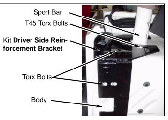
d. Using kit **driver side reinforcement bracket** as a template, mark the back body wall with center punch as shown.
