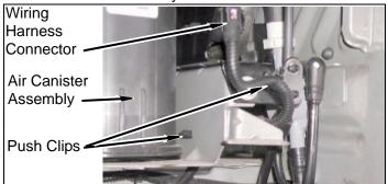
e. Carefully slide a small and large clip outward and remove a small and large vent line from air canister assembly and vehicle.
