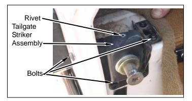
c. **All Models:** Drill rivet, and remove striker post, shims, and flat nut from tailgate striker bracket.
