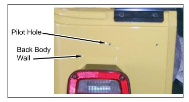
i. Install kit **striker plate** on back body wall and kit **reinforcement bracket** with a kit **bolt** (3/8" x 1") and a kit **flange nut** (3/8"). Tighten six torx bolts and two kit **bolts** (3/8" x 1").
