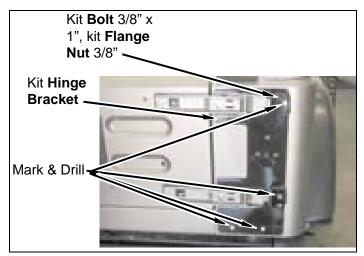
I. **TJ Models:** Install kit **hinge bracket** on body with a kit **bolt** (3/8" x 1"), kit **thick washer** (1/2"), and a kit **flange nut** (3/8"). Snug but do not tighten bolts at this time.
