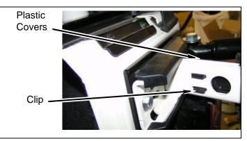
b. **2004 models:** Slightly twist the upper edge and remove two upper and lower plastic covers from the body side of the hinges.
