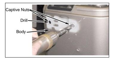
b. Position kit **passenger side reinforcement bracket** on body.
