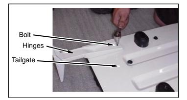
e. Install two kit tailgate hinge plates and tailgate hinges on tailgate.
