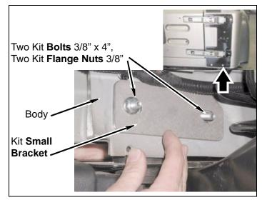
n. YJ Models: Install kit lower support bracket on body and kit hinge bracket with two kit bolts (3/8" x 1") and two kit flange nuts (3/8"). Do not tighten.
