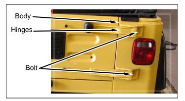
d. Position tailgate on the ground. Remove four bolts and tailgate hinges from tailgate.
