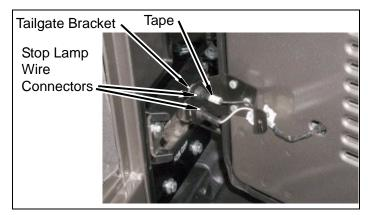
c. Remove grommet and wire harness from tailgate.
