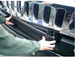
2. Remove 4 factory bolts, 2 on each side.
