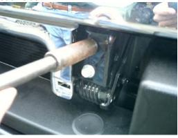
3. Install brush guard with the 4 factory bolts.
