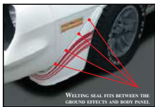
WETTING SEAL FITS BETWEEN THE GROUND EFFECTS AND BODY PANEL.
