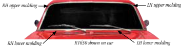
RH upper molding LH upper molding RH lower molding R1650 shown on car LH lower molding
