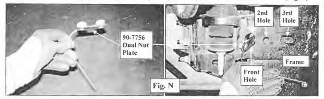
Step 17: Install the upper support plate (93-7608 Drvr and 93-7609 Pass) from the outside behind the core support, and secure the rear of the plate to the dual nut plate (90-7756) through 2nd & 3rd holes in the frame rails using the (2 per side) supplied 1/2" X 1 1/2" bolts and washers. Leave bolts loose at this time. (Fig O)
