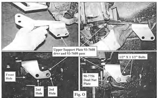
Step 18: Secure the front of the upper support plate (93-7608 Drvr and 93-7609 Pass) to the holes in the top of the winch plate (93-7610) using the (2 per side) supplied 1/2" X 1 1/2" bolts and hardware. (Fig P)
