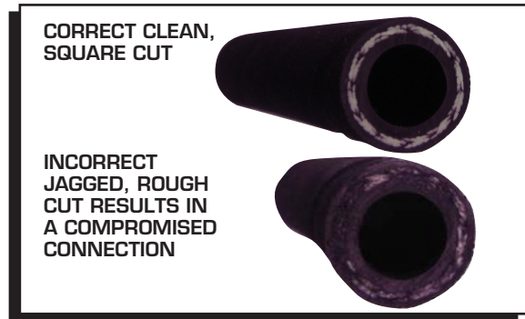
Figure 5 Severing the Hose Properly.
