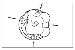
2. Turn the battery compartment so you can see one screw on each side. Remove all four screws with a small screwdriver.
