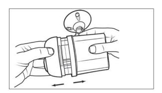
1. Remove front cover of Spotlight by rotating counter-clockwise as shown above. Pull face out from cup to reveal battery compartment.
