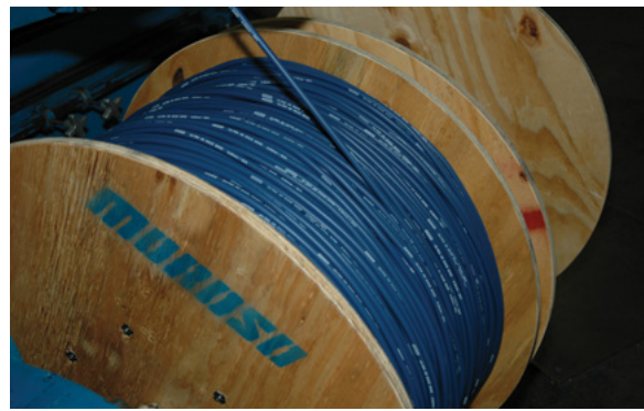
In the last step in the manufacturing process, completed wire is rolled onto wooden spools. Each spool holds 5,000-feet of wire awaiting the final steps to complete a length of spark plug wire.
