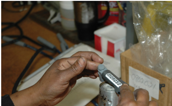
Moroso Ultra 40 Race Wire Sets receive a fiberglass reinforced silicone outer sleeve which requires a heat shrink sleeve at the boot in order to seal off the whole assembly.
