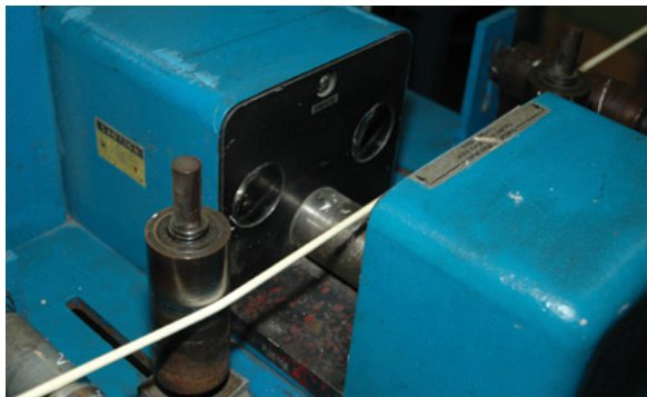
An optical laser measuring device keeps constant measurement on the completed wire as it comes to the end of the line. The machine operator must maintain the measurement within a specified amount and adjust as necessary.
