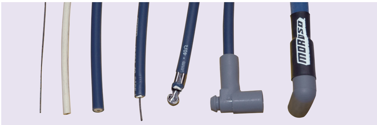
The manufacture of Ignition Wire requires several different steps: first, the center conductor (1) has EPDM (Ethylene Propylene Diene Monomer) rubber material formed around it (2). The wire is then re-fed into the machine where the outer silicone covering is formed and printed with the type of wire it is (3). The completed wire is then stripped back (4) and the terminal ends are crimped on (5). The plug boot is installed (6) and finally, for race applications, a silicone-jacketed fiberglass sleeve is slipped over the assembly and a shrink sleeve installed (7).
