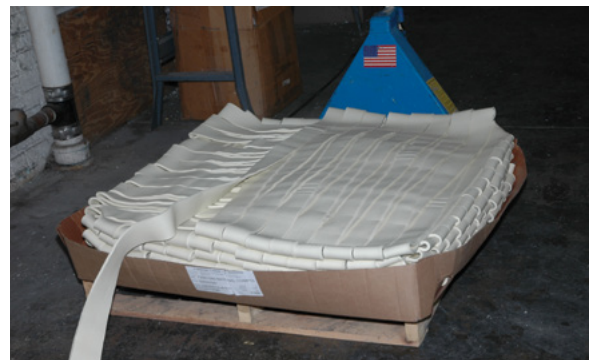
The rubber cover material for the center conductor starts out in this ribbon-like form. It's fed into a tube that heats and feeds it through a series of collets to form it around the center conductor.
