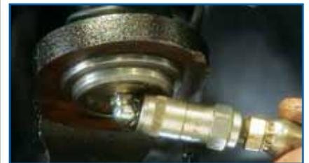
When greasing MOOG chassis parts, a hand grease gun is preferred. If a pressurized grease gun is used, take great care that you don't overfill the boot, which may cause it to tear.
