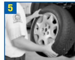
5 Replace tire/wheel on vehicle. Lower vehicle to ground and torque lug nuts to specification, using a torque wrench.
