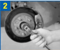
2 Remove axle nut, using an axle nut socket. (An impact wrench is not recommended.) Socket size can range from 30mm to 36mm.
