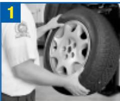
1 Raise vehicle off the ground and remove lug nuts and wheel.
