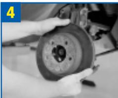
4 Remove the brake rotor.
