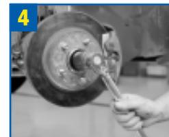
4 Torque axle nut to manufacturer's specifications. Do so while vehicle is raised and hub assembly is unloaded. Replace with new axle nut. Do NOT use an impact wrench.
