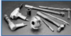
Tools required for proper removal and installation of wheel end modules.
