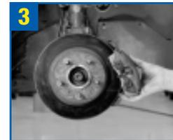
3 Reassemble brake rotor and caliper.
