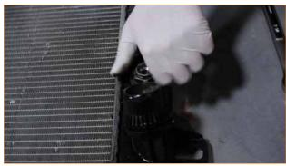
**4.** Reconnect the radiator to the intercooler. The bolt nearest to the cold side intercooler outlet will need to be replaced by the Mishimoto supplied M8 X 1.25mm bolt and washer. You can reuse the factory hardware for the other three mounting locations.
