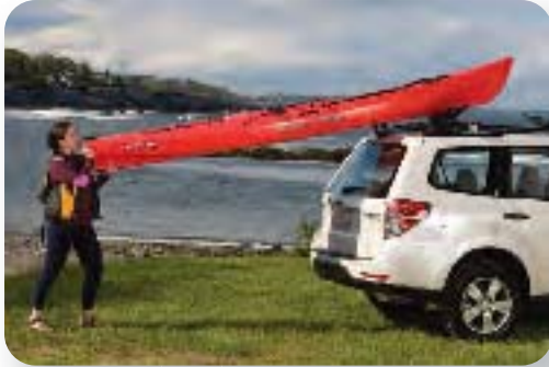
Extend the Loading Frame. Set the front of the kayak into the V-Block. Slide the kayak up and into the carriers.
