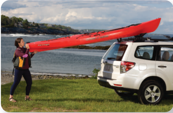
Extend the Loading Frame. Set the front of the kayak into the V-Block. Slide the kayak up and into the carriers.
