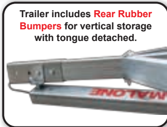
Detachable Tongue to Lower Storage Space Requirements
