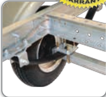
400 lb Capacity Leaf Spring Suspension
