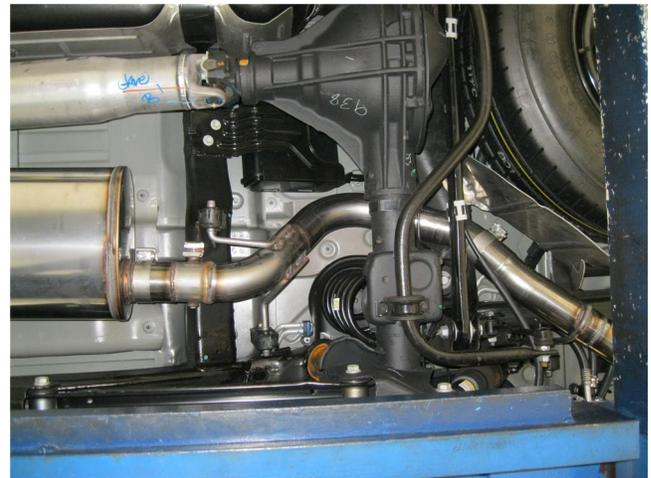
**Step 3.** Complete the initial installation by attaching the Extension Pipe Assembly (containing the exhaust valve) to the Muffler and the Resonator/Tailpipe Assembly using the supplied 3.00" clamps.
