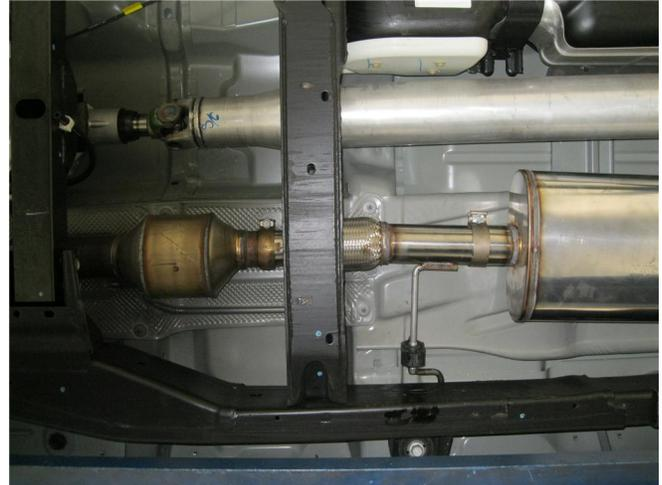
**Step 2.** Begin installation of the new system by attaching Inlet Pipe Assembly at the ball flare using the OEM clamp and fitting the hanger into the rubber insulator. Next attach the muffler to the inlet pipe using a supplied 3.00" clamp. Leave all clamps loose for final adjustment of the complete system.
