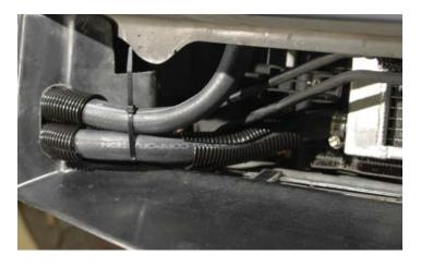
249. Inspect your hoses carefully and notice any areas that need additional protection, such as the swing arm mounting bracket, other hose clamps, etc. Protect any such areas using the provided split loom.
