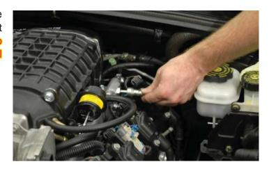
170. Secure the fuel line using the lock clip. Make sure that the lock clip snaps into place.
