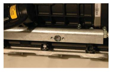
125. Install the fuel manifold using a 10mm socket and torque wrench. Torque the manifold fasteners to 106 in-lbs.
