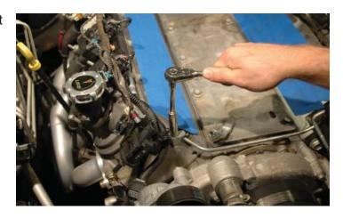
46. Remove the coolant vent pipe. Ensure that the O-ring gaskets under the vent pipe blocks do not stick to the cylinder heads. If so, remove them as new gaskets are supplied.
