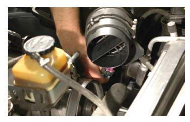
63. Unscrew the three screws holding the cover of the airbox to the housing. Pull up on the cover and remove for later reinstallation.
