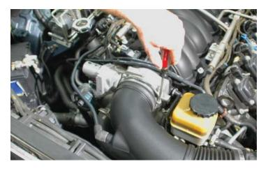
17. Remove the PCV tube from the air tube and from where it connects to the valve cover barb.
