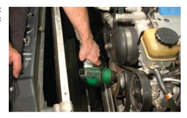
82. Install the provided drill guide and bolt at the harmonic damper on the crank pulley.
