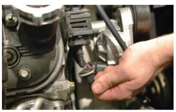
21. Remove the other end of the EVAP line from behind the throttle body on the driver side manifold.
