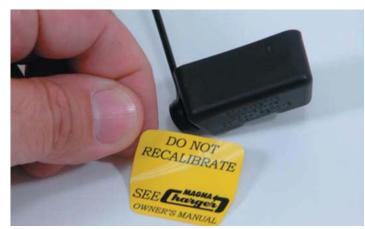
274. Locate the OBD II connection plug along the bottom edge of the dash above the brake pedal. Install the OBDII cover on the port and secure the attached cord around the wiring harness behind the port. Push the cord up behind the instrument panel so it will not interfere with the vehicle operation.
