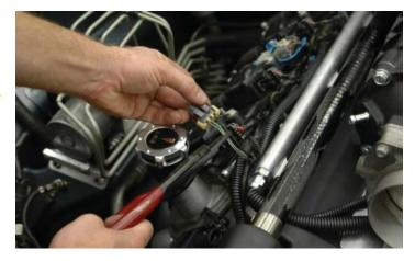
White, Green and Black wires using the crimp/shrink connectors supplied. The new harness wires are all white, so care must be taken so the new white wires are in the same positions as the colored wires on the original connector. It's a good idea to stagger your connections to avoid bulges in the split loom. Strip about ¼" of insulation from the ends of all the wires and crimp the connectors on.
