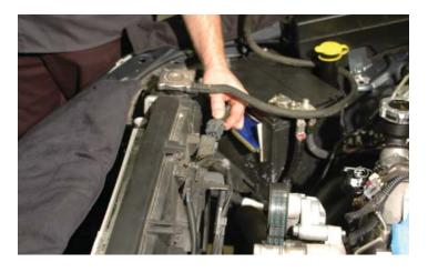
69. Remove the fan shroud from the radiator by releasing the lock tabs on each side of the fan shroud and pulling free.
