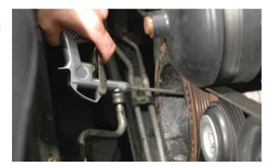
86. Use the provided reamer bit to clean and hone the holes you just drilled.
