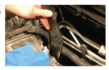
60. Vehicles with automatic transmission only. Manual transmission vehicles please skip to step #62. The automatic transmission fill tube will need to be moved slightly outward to avoid contact with the supercharger fuel cross-over pipe.
