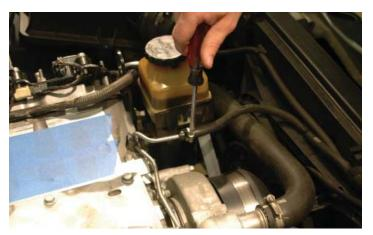
45. Remove the coolant vent pipe attachment bolts with a 10mm socket wrench.
