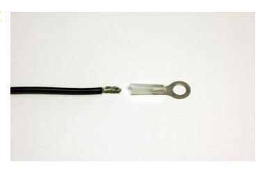
260. Connect the **Black ground negative** (-) wire of the Fuel Pump Booster onto the chassis ground connection located just below the Cruise Control module platform. Remove the nut with a 10mm wrench and place the ring terminal on the stud. Re-install the nut and tighten it securely.
