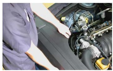
15. Use a 7mm nut driver or flat-blade screwdriver to loosen the Air Tube clamp at the Mass Air Flow meter (MAF).
