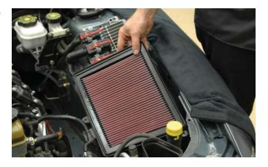
178. Replace the air box cover, tighten the three fasteners and place the K&N "Warning" label on the cover. This label stops a mechanic/technician from removing the high flow K&N filter which is reusable using a K&N filter service kit.
