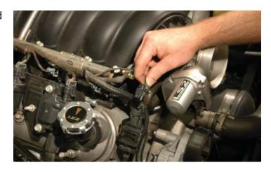
26. Remove the PCV hose that connects the intake manifold to the engine valley cover vent.
