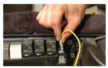
211. Remove the nut of the chassis ground connection located just below the Cruise Control module platform (below and to the rear of the fuse center) with a 10mm wrench and place the ring terminal on the stud.
