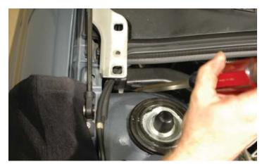
262. Cut the Tie-strap at the bottom of the "drop" tab covering the wires where it meets the Fuse/Relay center. Cut the adhesive wrap at the center of the tab and pry off each to each side. Using a small straight blade screwdriver, gently pry the locking tabs free of the upper cover of the conduit to free the cover. Care must be taken because it would be easy to snap off the tabs.
