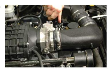
184. Install the PCV inlet hose. Cut a 17" length of 3/8" hose supplied and attach one end to the barb near the front of the passenger side valve cover by the oil fill neck. Attach the other end of the hose to the barb on the side of the new air tube. No clamps are necessary.
