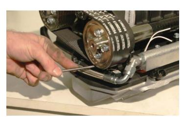
124. Install the fuel manifold O-ring into the recess on the fuel rail with some of the grease supplied.
