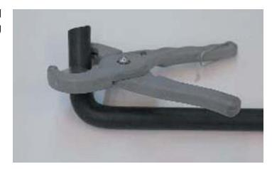
243. Connect the short "elbow" end of the hose to the inlet barb on the intercooler pump as shown. Route the other end up toward the reservoir.
