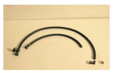
159. Connect the long EVAP hose with the Test port fitting to the fire wall connection.
