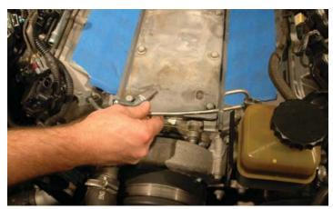
47. Install the new vent pipe O-ring gaskets using the supplied Lubriplate lubricant to hold them in place.
