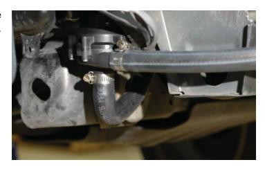
244. Secure the long end of the "elbow" hose to the bottom reservoir barb using a provided #10 hose clamp, tighten firmly.
