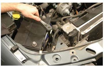
196. Completely remove the battery from the vehicle. Put aside for later re-installation.
