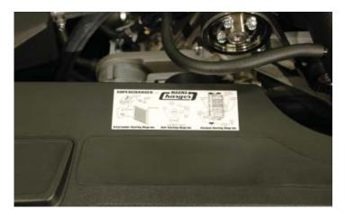
277. Start the vehicle for 5 seconds and shut off, once again check for fuel leaks and supercharger belt alignment. Test drive vehicle for the first few miles under normal driving conditions, listen for any noises, vibrations, engine miss fire or anything that does not seem normal. The supercharger does have a slight whining noise under boost conditions, which is normal. Check intercooler reservoir as needed.
