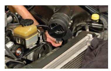
180. Here is the new air tube and mounting components.
