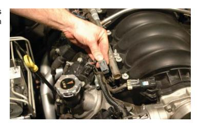
28. Remove the injector harness clips from the intake manifold by pulling the clips from the fuel rail mounting holes.
