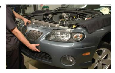
252. First loosely replace a couple of the upper mounting screws to hold the unit from falling.
