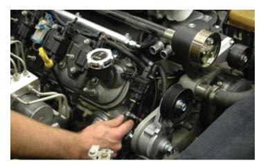
163. Connect the remaining end of the short EVAP hose to the fitting on the passenger side of the inlet manifold above the supercharger drive shaft as shown, no clamp is necessary.
