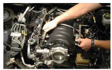
39. Use a shop vacuum cleaner to remove any debris or dirt from the intake port area and engine valley cover.
