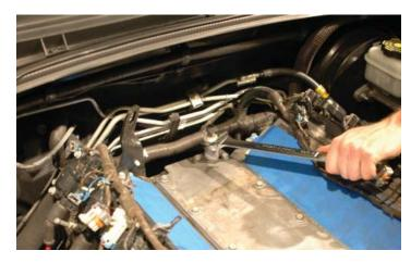
51. Remove the engine valley cover and gasket by removing the eleven bolts with a ratchet and 13mm socket and lift the cover free.
