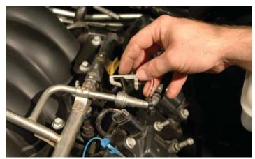
35. Use the supplied removal tool to remove the fuel line connector. First push the line onto the barb, insert the fuel line removal tool and press it into the fuel line, then pull on the fuel line to separate the fuel line from the hard line barb. Catch the dripping fuel with a shop rag and be sure to dispose of properly. We suggest you put a cap on both the fuel line barb and plug the end of the hose to avoid further contamination and mess.
