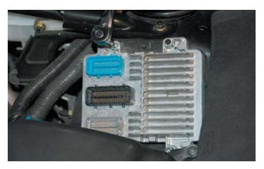
5. Note: If your vehicle has an automatic transmission, you will also need to remove the transmission control computer located on the back side of the drivers kick panel, inside the vehicle.
