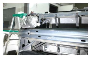
240. Cut a piece of the supplied ¾" hose to 24" in length. Connect one end of the hose to the lower barb of the heat exchanger. Secure the hose with one of the provided #10 hose clamps and tighten firmly. Route this hose through the same hole, below the hose just installed.
