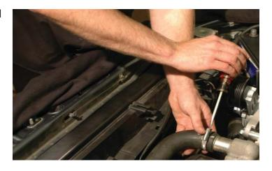
177. Replace the stock filter element with the K&N air filter element supplied.
