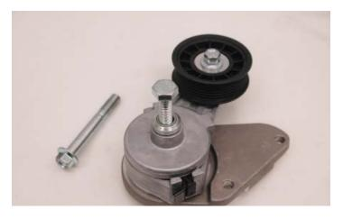
97. Assemble the tensioner with the adjustable bracket brace as shown. Test fit the tensioner assembly, and adjust the bracket brace as needed.
