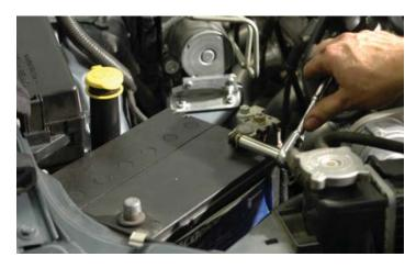
195. Use a 13mm socket to remove the battery hold down bracket as shown.
