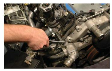
95. Relocate the bolt and ground wire to the existing hole just under the existing freeze plug as shown. Tighten the bolt with the ground wire incorporated using a 13mm wrench.
