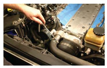
68. Unplug the fan control plug at the passenger side of the fan shroud.
