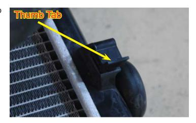
80. Carefully lift the radiator free from the vehicle.
