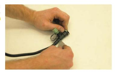
158. Use the piece of 5/16" EVAP hose supplied and cut it into two pieces. One piece 32" long and the other 17" long. Starting with the longer of the two, assemble the hose with the test port on one end (the right angle will go on the other end after the hose is routed), use the #6 clamps supplied. On the remaining hose, assemble it with the straight quick disconnect fitting and clamp as shown.
