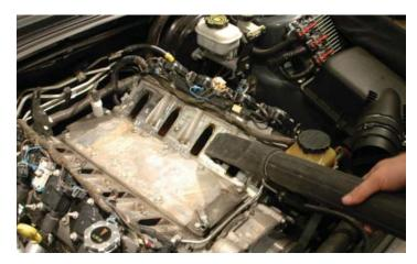
40. Use alcohol or a suitable solvent to wipe the heads clean being careful to not allow any debris to fall into the exposed ports.
