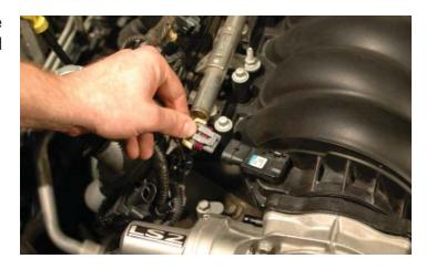
30. On both sides of the engine disconnect the ignition coil pack connectors from the coil packs by first removing the blue lock key.
