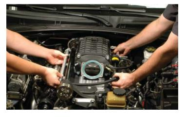
129. Remove the split-loom sections that support some of the manifold to cylinder head bolts. Start all ten bolts by hand to ensure proper alignment of the manifold.
