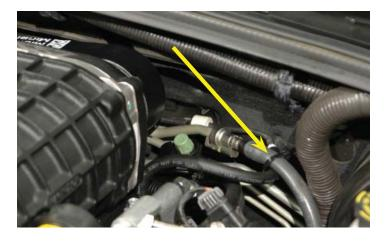
169. Connect the fuel line to the fitting on the fuel manifold. Pull on the fuel line to ensure that it is securely attached. You should not be able to remove the line without using the fuel line removal tool.
