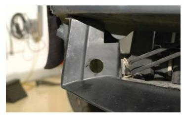
229. Drill a second hole of the same size above the hole you just made, also using either a sharp knife or hole-saw as shown.
