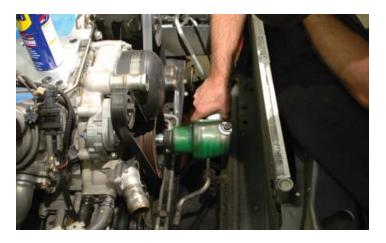
88. Blow out the holes that you created again, being sure you are wearing safety glasses and that no debris contaminates any openings.
