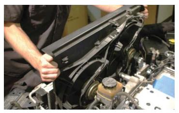
105. Press the AC condenser back onto the radiator mount tabs. Press on the ends of the assembly, not in the center tube-fin sections where the heat exchanger could collapse.
