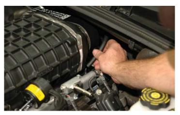
168. Use a loose zip tie to anchor the vacuum hose to the existing fuel line hose as shown.
