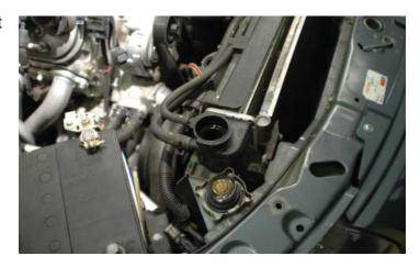
44. Remove the coolant vent hose from the vent pipe.
