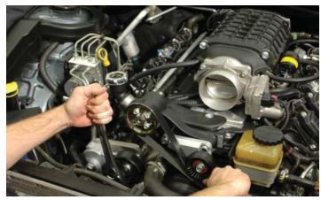
176. Reconnect the upper radiator hose and tighten the clamp in position beyond the barb.
