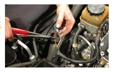
140. Pull the cut end of the remaining wires back out of the split loom to the loom junction near the power steering reservoir on the driver side of the engine.
