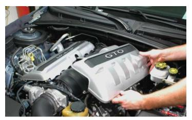
13. Use a flat blade screwdriver to pry up on the five push pin rivets on the radiator cover.
