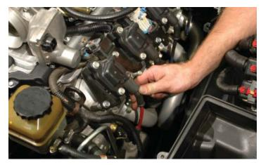
137. Plug in the main coil pack control connector and blue lock keys on both sides of the engine.
