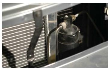
235. Install the two 6 X 20mm bolts through the power steering cooler bracket and into the lower brackets on the heat exchanger. You can access these bolts through the lower grill or by pulling down the lower splash apron. Tighten the two bolts securely with a 10mm socket wrench.
