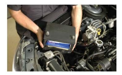
226. Tighten down the battery hold-down bracket using a 13mm wrench.
