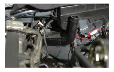
221. Reattach the rear mounting bolt of the reservoir to the original existing threaded hole on the frame rail using the stock bolt as shown.
