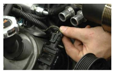
165. Locate the Vacuum accessory line at the fire wall on the passenger side by the heater hoses.
