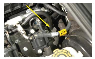
187. Route the hose forward between the fuel rail and coil bracket.
