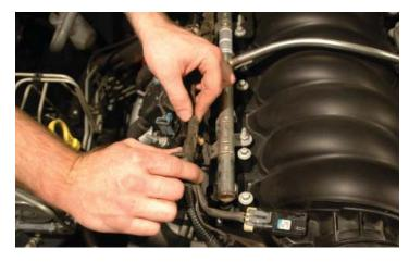
29. At the front of the intake manifold locate the Manifold Absolute Pressure (MAP) sensor and disconnect the electrical connector.
