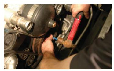
91. Install the new harmonic damper crank bolt and torque to General Motors specifications of 50 N-m (37 ft lbs) then tighten an additional 140° using a torque angle meter.
