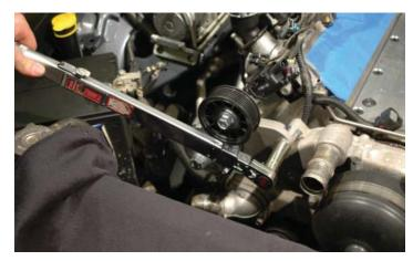
99. Torque the main tensioner bolt to 50 ft lbs locking against the nut on the adjustable bracket brace.
