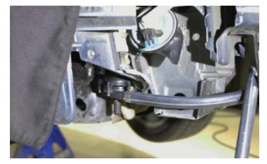
242. Trim the molded 90° "elbow" hose supplied by cutting 1-1/4"" from the short leg and the long end to 24" in length.
