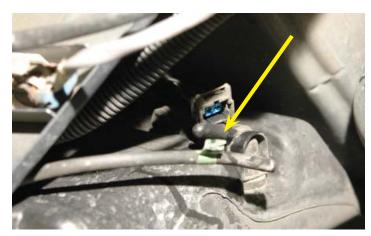
199. Locate and remove the bolt that secures the side of the reservoir bolt with a 10mm socket wrench. This bolt is near the horn relay on the cross frame.
