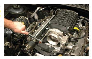
132. Plug in the injector control plugs on both sides of the supercharger assembly.
