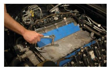
52. The gasket will be reused, the original valley cover and bolts will not. Inspect the gasket for any damage and then reinstall, note that it will only fit correctly in one position.
