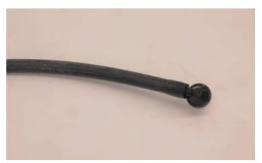
191. Install the check valve into the grommet on the brake booster. Route the hose over the reservoir, forward between the fuel rail and coil bracket (parallel to the PCV hose just installed) as shown.
