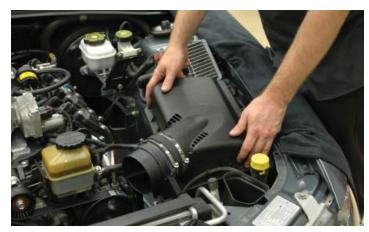
179. Plug in the MAF electrical connection to the MAF Sensor on the bottom of the air tube on the air box cover as shown.
