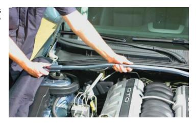
12. Remove the two engine covers by pulling up firmly along the edges.
