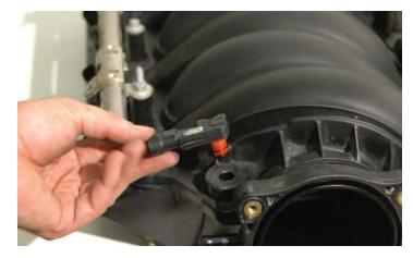
122. Apply a small amount of the grease supplied to the MAP sensor seal and install the sensor in its new location at the right rear of the supercharger manifold.
