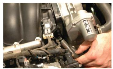
27. Disconnect the eight fuel injector connectors by pulling up on the grey release latches and then squeezing them at the top.
