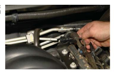
24. We will not be using the OEM EVAP lines, but we will be utilizing connectors, so put them aside where they won't get damaged for later usage.
