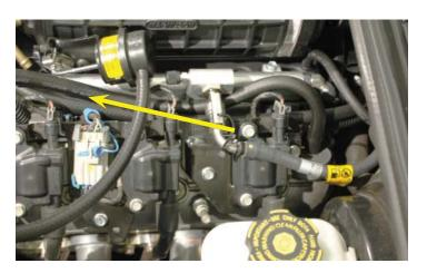
188. Install the plain end of the 16" PCV outlet hose on the forward barb of the supercharger inlet on the driver side of the inlet as shown.
