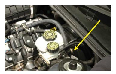
192. Connect the end of the brake booster hose to the remaining barb on the driver side of the inlet manifold as shown.
