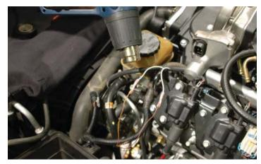
147. Ensure that the split loom reaches all the way to the supercharger lid and cut the split loom to fit. Use tape to join the split loom to the existing wire harness as shown.
