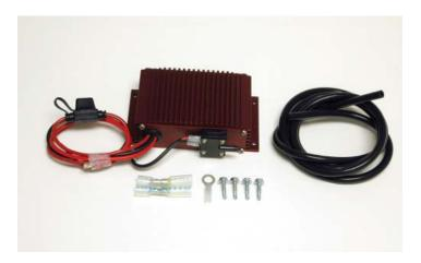
258. Remove the FUSE/RELAY center cover and using the Fuel Pump Booster as a template, drill two 3/16" holes along the top edge to mount the Fuel Pump Booster unit. Assemble the Fuel Pump Booster to the Fuse/Relay center cover with the screws provided. Replace the cover with the fuel Pump Booster attached on to the Fuse/Relay center.
