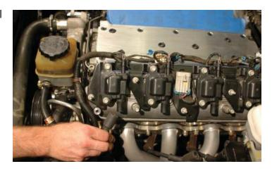
110. Use a 10mm wrench to unbolt the coil brackets from both sides of the engine.
