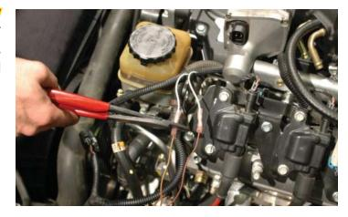
146. Use a heat gun or a hair dryer set on high to shrink the insulation on the connectors so that they contract around the wires completely. You must shrink the insulation, as crimping the connectors alone is not enough to secure them!
