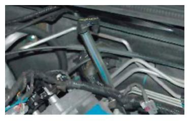
61. Move the automatic transmission fill tube by pulling it firmly outward towards the fender of the vehicle. It will only be necessary to move the tube 1/4"- 3/8". After installing the supercharger and manifold assembly, check for contact between the transmission fill tube with the fuel cross-over pipe, and the brake lines. See step #155.
