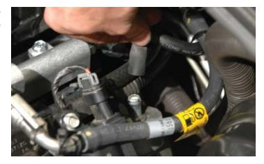
186. Assemble the PCV outlet hose by cutting a 16" length of the 3/8" hose. Attach one end the hose to the driver side valve cover PCV barb.
