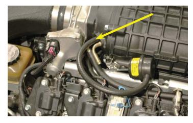
189. Remove the brake booster check valve from the OEM hose from the factory manifold.
