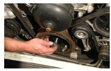
83. Torque the provided bolt on the drill guide to 35 ft lbs. Verify your torque wrench settings.
