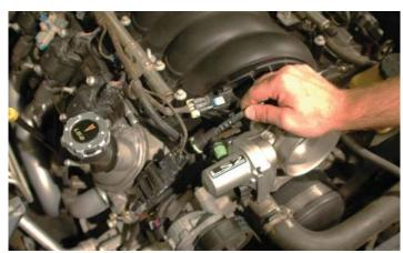
23. Remove the other end of the EVAP line at the fire wall by squeezing on the connector and pulling it free.
