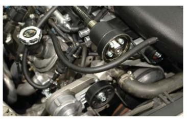
185. Remove the rubber cap from the rear of the driver side valve cover hose barb just beyond the coil brackets.
