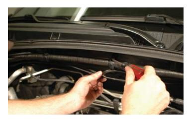
115. Remove the harness clamp from the fire wall, it will not be re-used.
