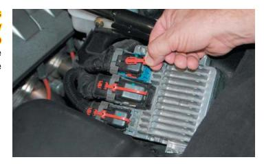
2. There are three computer connectors, Grey, Black and Blue. Remove the connectors by first removing the Red locking key, then pushing in on the Black cover and pushing the Grey latch down to open it.
