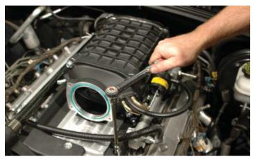
131. Install the throttle body onto the new inlet manifold with the original mounting bolts. Note that the throttle body control is on the driver side of the supercharger to clear the jack shaft. This will not affect function. Torque the mounting bolts to 106 in-lbs.
