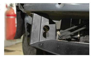
230. Connect the two holes as shown using a sharp knife to remove the material between. Then sand or ease the hole to remove any sharp edges in the plastic.
