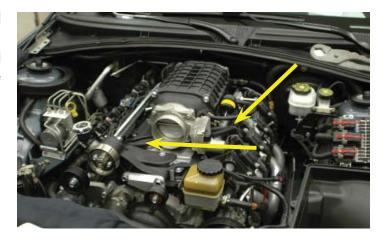
161. Install the right angle fitting on the end of the routed hose, secure with provided #6 clamp and connect to the top barb of the Purge solenoid.
