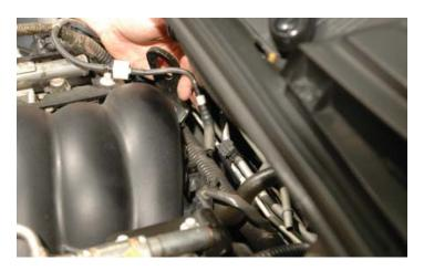
32. Relieve the pressure in the fuel system by removing the cap.
