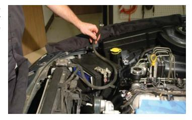
66. Disconnect the radiator overflow hose from the barb at the radiator fill neck, unclip from the fan shroud mounting clips and pull the hose free, tuck the hose into the air box out of the way.
