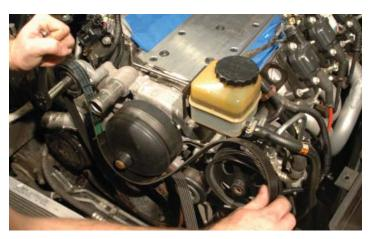
93. Use a 13mm wrench to remove the OEM tensioner assembly.
