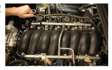
38. Remove the intake manifold, fuel system and throttle body assembly. CAUTION! Make sure that you do not drop any debris into the intake ports!
