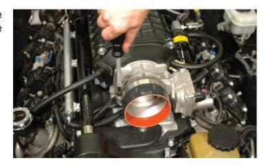
182. Attach the bellows end of the air tube on the air meter.
