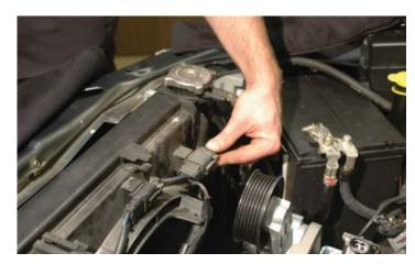
107. Reconnect the radiator over flow hose and snap into the guide clamps along the fan shroud.
