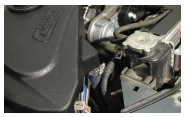
245. Route the long ¾"hose end from the heat exchanger upper barb up into the engine compartment and connect it to the rear barb of the water manifold as shown. Secure the hose with #10 clamps.
