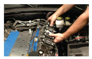
112. Remove the plastic wire covers from both coil brackets using a small flat head screwdriver to release the clips holding the halves together.
