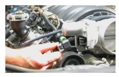
20. The EVAP Solenoid is located at the front of the passenger side cylinder head. To disconnect the EVAP line, press the gray tab and pull to remove.
