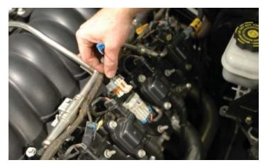
31. Remove the vacuum accessory hose and connector from the rear of the manifold.
