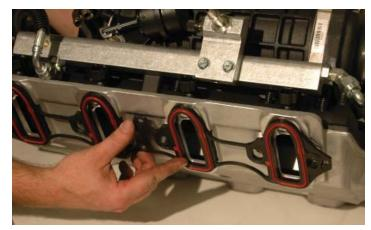
127. Remove the tape from the ports. Use silicone or some mild soap and water solution to lubricate the port surfaces. This will help align the manifold and bolt holes. (Do not use anything that will damage the silicone port gaskets.)
