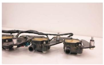
135. Mount the prepared driver side coil pack to the valve cover using the supplied hardware. Torque the mounting bolts to 106 in lbs. Verify your torque wrench settings.
