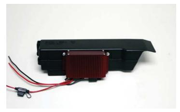
259. Connect the Ring connector to the **BLACK** Ground wire negative (-) by stripping a 1/4" of the insulation from the end of the wire and crimping it on securely.
