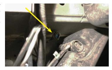
198. Remove the fluid supply hose from the pump and then temporarily cap the pump nipple with the rubber cap supplied. Some fluid may leak out, so have a towel or shop rag handy and make sure to dispose of properly.
