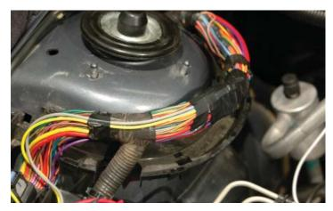
267. Carefully tuck all the wire back into the conduit and snap the top cover back into place. Snap the conduit mounting tabs back onto the shock tower securing the assembly. Route the new RED wires out at the base of the conduit.
