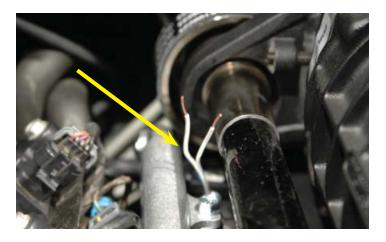
142. Cut the supplied white wire in half. Strip off about ¼" off the four ends of the white wire. Use two crimp/shrink connectors to join the IAT wires together extending their reach.
