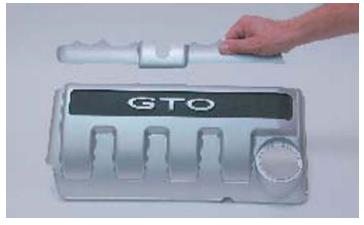
280. On the left side engine cover trim the cover as well. A little more care must be used on trimming this cover as you must make room for the bypass canister. Trim and test the cover fit several times to get a good fit and finish. Leave the finished covers off the engine until you have completed your test drives and final inspection.
