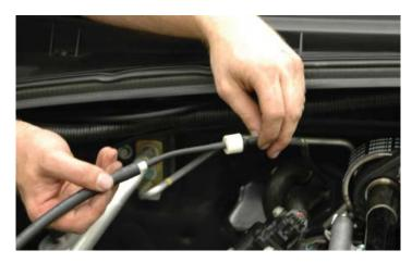
167. Remove the cap from the small barb on the driver side, rear corner of the supercharger lid. Connect the new extended vacuum accessory line to the now exposed hose barb.
