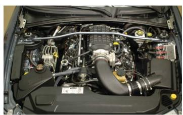
278. After the initial test drive gradually work the vehicle to wide open throttle runs, listen for any engine detonation (pinging). If engine detonation is present let up on the throttle immediately. Most detonation is caused by low octane gasoline still in the tank.
