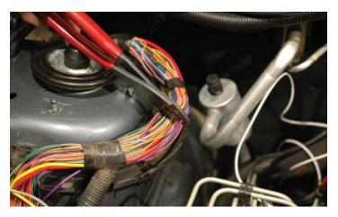
264. Using the Crimp/Shrink connectors supplied, connect the RED WIRE WITH THE FUSE HOLDER from the Fuel Pump Booster to the end of the PURPLE wire that goes to the Fuse/Relay center. Connect the RED without the fuse to the end of the PURPLE wire that goes toward the fire wall.
