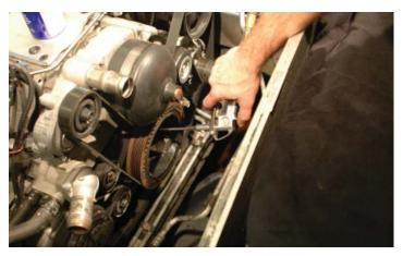
89. Put a bead of Green Loctite on the two provided hardened crank pins and insert them into the holes you just prepared.
