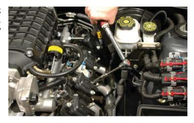
136. Reinstall all plug wires on both sides of the engine.
