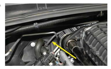
166. Remove the short piece of hose from the coupler (hose mender) beyond the check valve, and install the supplied longer length of 3/16" hose onto the end of the coupler (hose mender).
