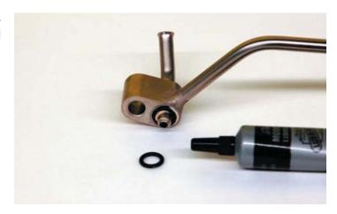
48. Install the new vent pipe with the OEM bolts and torque them with a torque wrench and 10mm socket to 106 in-lbs. Verify that your torque wrench is set to in-lbs!
