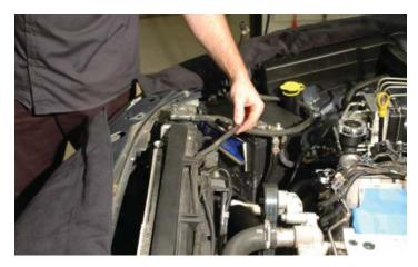
67. Disconnect the upper radiator hose from the water pump barb and tuck the hose between the block and the airbox on the driver side out of the way.
