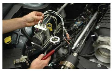
151. Use a heat gun or hair dryer set on high to shrink the insulation so that it contracts around the wires completely. You must shrink the insulation, as crimping the connectors alone is not enough to secure them!
