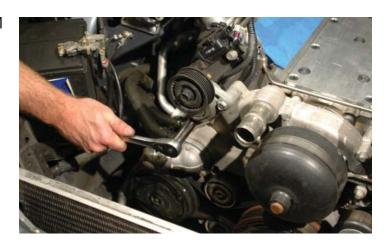
94. Use a 13mm wrench to remove the ground bolt on the passenger side head.
