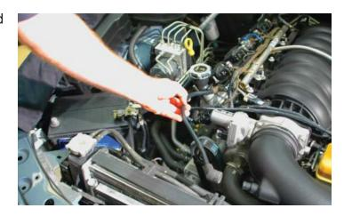
18. Remove the air tube completely, it will not be re-used.
