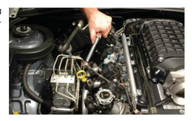
134. Pre-mount the supplied spacers using the provided grommets to hold the bolts in place on the driver side coil pack as shown.
