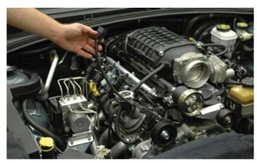
173. Route the extended harness under the supercharger, behind the idler support bracket and plug the connector into the throttle body as shown.
