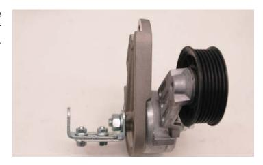
98. Torque the tensioner mounting bolts to 40 ft lbs. Verify your torque wrench settings.
