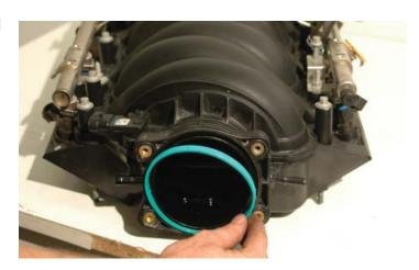
120. Install the throttle body O-ring into the groove on the new inlet manifold. The LS2 throttle body will be installed after the supercharger assembly is installed on the engine.
