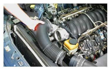
19. Disconnect the Electronic Throttle Control (ETC) connector on the passenger side of the throttle body.
