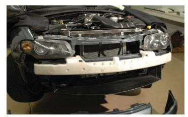
251. Re-place the fascia by carefully lifting the unit into position.
