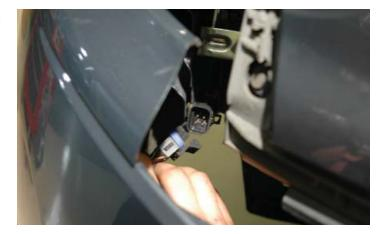
254. Snap the locking tabs back into place below the headlights and then replace the remaining mounting screws and tighten all around.
