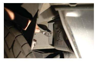
201. Remove the push-lock fastener that secures the bottom of the reservoir to the wheel well.
