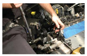
100. Use a 15mm wrench to tighten the brace bracket bolt on the passenger side head where the ground wire was removed in step #94.
