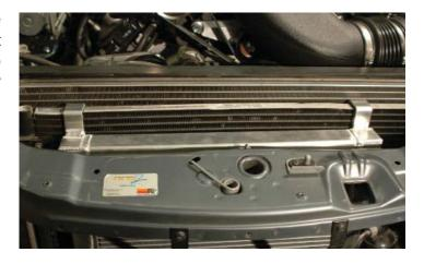
234. Verify that you have adequate clearance between the black A/C dryer cylinder and the heat exchanger. If there is any question, loosen the dryer cylinder mounting bolt and rotate as needed...be sure to re-tighten the mounting bracket bolt.
