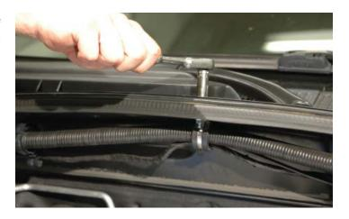
118. Remove the throttle body by removing the four mounting bolts with a 10mm socket wrench.
