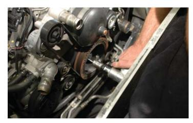
87. Use a 15/16" (24mm) socket and impact wrench to remove the temporary bolt and drill guide tool installed in steps #82 and 83.
