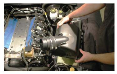
64. Remove the OEM air filter.
