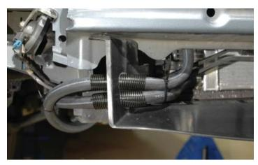
248. Cut pieces of the supplied split loom to protect your hoses from any existing hard edges or potential wear points such as the transmission cooler hard line.
