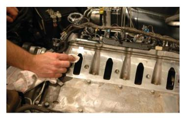
41. Cover the intake ports with tape or clean rags to keep dirt and debris from entering the engine.
