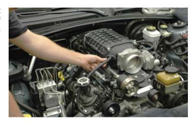
164. Connect the electrical control plug to the EVAP Solenoid.
