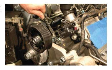
101. Tighten the two adjustable bracket bolts.
