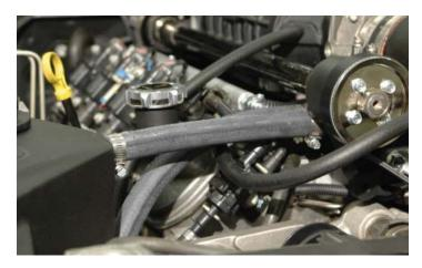
247. Cut two pieces of the supplied split loom to cover the hoses as they pass through the air deflector. Loosely group your hoses together using the supplied zip ties.
