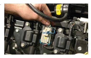
138. Remove the two rocker cover socket pins on the driver side and reinstall incorporating the supplied spacers. Tighten down using a 10mm wrench. These spacers are only necessary on the driver side.
