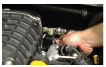
160. Route the other end of the hose forward between the driver side coil pack and the fuel rail. Pass the hose under the inlet manifold and supercharger drive toward the EVAP purge solenoid.
