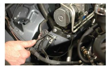
212. Add the **Black** ground negative (-) wire with the ring terminal to the chassis ground connection and re-install the nut to the ground.
