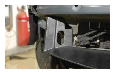
231. Cut two strips of the supplied adhesive backed rubber about 4" in length. Assemble the supercharger intercooler heat exchanger by peeling the backing paper off the two short plastic strips and apply them to the inside of the upper mounts of the heat exchanger.
