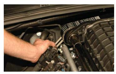
155. If you have an automatic transmission: Ensure that there is clearance between the transmission fill tube, the fuel cross-over pipe, and brake lines. Cut a piece of the provided 3/16" hose to protect the lower brake lines. Split the hose lengthwise and slip over the brake lines where they are adjacent to the transmission fill tube. This was referenced in steps #60-61.
