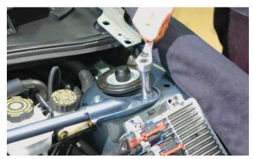
11. Remove the strut tower brace and fasteners from the vehicle, the brace can be reinstalled after the supercharger installation.
