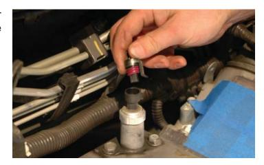
50. Remove the engine oil pressure sensor from the valley cover with a 1-1/16" wrench.
