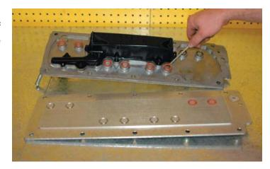
54. Install the new engine valley cover and flathead bolts supplied with a 5mm Allen socket and torque the bolts to 18 lb-ft.
