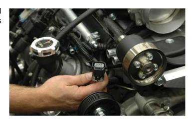
172. Plug in the supplied ETC extension harness into the existing ETC plug.
