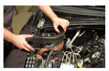
263. Once the conduit cover has been removed, locate the medium size solid **PURPLE** wire and cut it as shown. Make sure you are cutting the correct wire, there's only one that fits this description.
