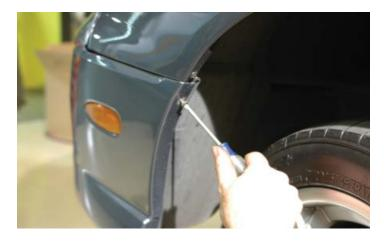
73. Carefully (do not use excessive force or you can break the plastic mounting tabs) pull out on the wheel well edge of the front fascia just enough to clear the lip. This picture shows it pulled further out since the clips were already unsnapped.
