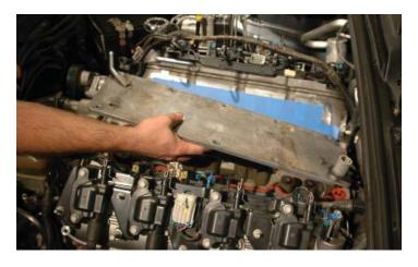
53. Using a small straight blade screwdriver, remove the eight O-rings from the underside of the engine valley cover and transfer them to the grooves in the bottom of the new cover.
