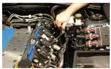
111. Remove both coil brackets from the engine.
