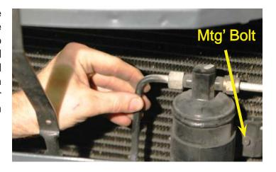
233. Lower the front heat exchanger into place on the front of the A/C condenser. Ensure that the adhesive backed rubber strips sandwich the existing A/C condenser and don't get pulled away from the mounting hooks.
