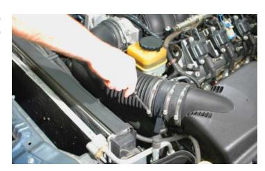
16. Use a 7mm nut driver or flat-blade screwdriver to loosen the Air Tube clamp at the throttle body.
