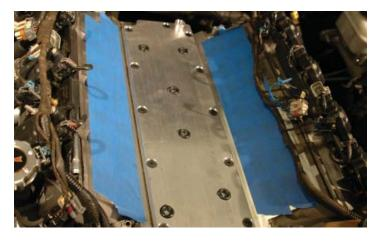
57. Use some Teflon tape or paste on the threads of the removed Oil Pressure transmitter and install the Oil Pressure Transmitter in the new valley cover with a 1-1/16" socket and torque it to 15 ft-lbs.
