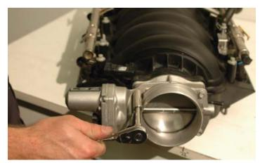
119. Carefully remove the original O-ring behind the throttle body on the original intake manifold.
