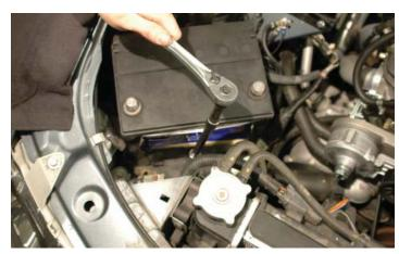
227. Re-attach the battery positive (+) terminal and tighten using a 10mm wrench.
