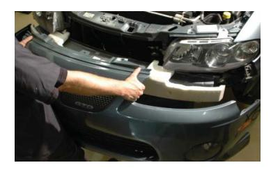
78. Remove the hard foam fascia backing by pulling it off the frame support.
