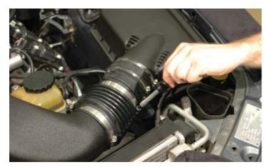
183. Attach the hose end of the air tube to the throttle body. Tighten all clamps securely.
