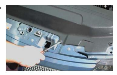
14. Lift up and remove the radiator cover and put aside for later re-installation.
