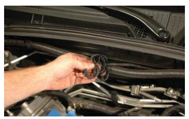
116. Here is the new harness clamp assembly, it will mount in the rain gutter hole that you removed the screw from in the previous step.
