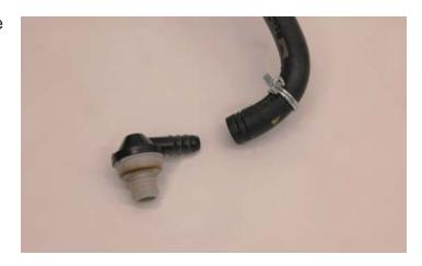
190. Cut a 22" long piece of the supplied 11/32" brake hose. Install the just removed factory check valve on one end of the hose.
