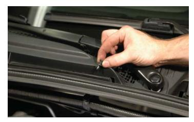
114. Using a small straight blade screwdriver, open the harness clamp and pull the harness free.
