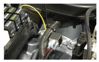
215. Install the Fuse/Relay center cover on the base by raising the relay slightly to hook the rear edge of the cover on the base then snap the cover in place.
