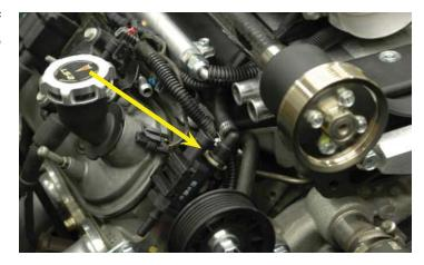
162. Connect the quick disconnect fitting from the shorter EVAP hose to the lower connection on the solenoid.
