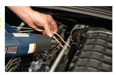
144. Slide a piece of the supplied split loom over the white wires. Route the wires under the fuel rail between the rail and coil brackets forward, and under the throttle body to the driver side of the vehicle.
