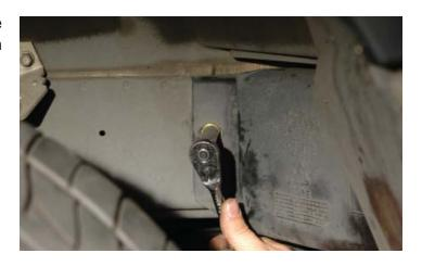
222. Secure the reservoir bottle with the stock fasteners using the stock bolt at the cross member (near the horn relay) into the bolt clip on the reservoir, and the push rivet to the wheel well.
