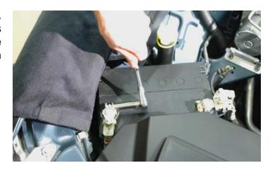
10. On top of each shock tower remove the two nuts that secure the strut tower brace with a 13mm socket wrench.
