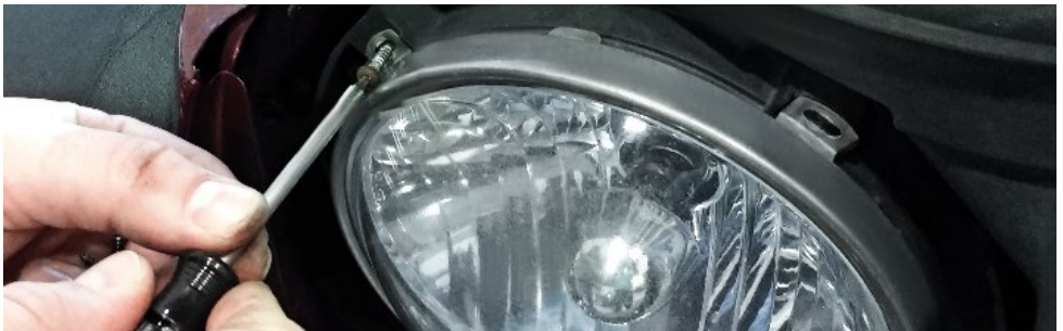
The headlamp bezel is held in place with 4 Torx screws
