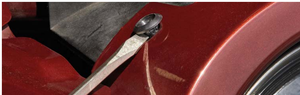
Use philips and/or flat blade screwdrivers to remote clips (clip design may be differ on your vehicle)
