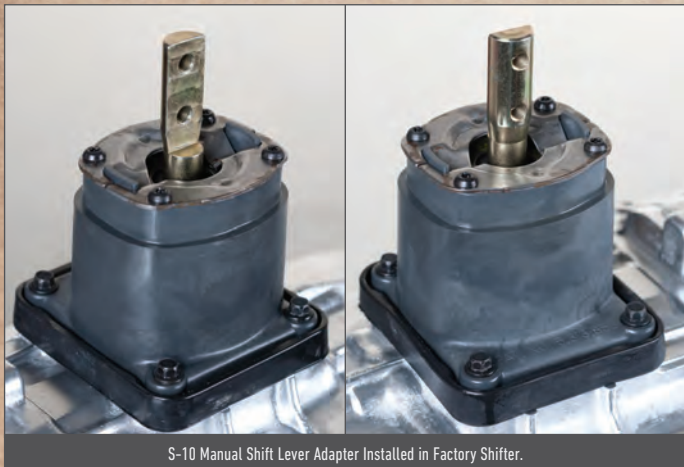
S-10 Manual Shift Lever Adapter Installed in Factory Shifter.
