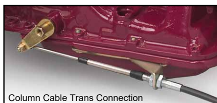
Column Cable Trans Connection
